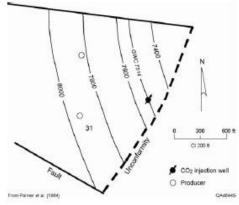
Figure 9. St. Elaine Bay field gravity-stable pilot run in a compartment bounded by faults and an unconformity.
