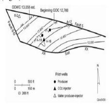
Figure 7. Weeks Island S sand gravity-stable pilot conducted in steeply dipping structure.
